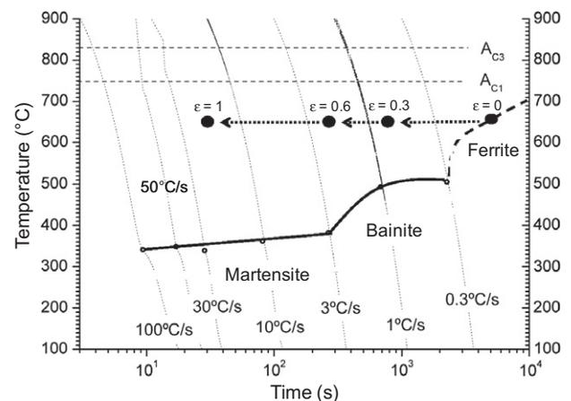
Fig. 1. Continuous cooling phase transformation diagram for a 0.26C–1.96Si–2Mn–0.31Mo (wt.%) steel. Solid circles represent the start of ferrite phase transformation for the steel deformed at different strains at 570  $^{\circ}\text{C}$  followed by isothermal holding at 650  $^{\circ}\text{C}$ , based on metallography observation.
