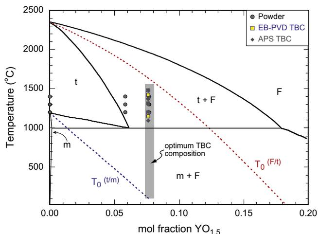
Fig. 1. Zirconia-rich portion of the  $\text{ZrO}_2\text{--YO}_{1.5}$  phase diagram, showing the concentrations and aging temperatures used in this study. Both the equilibrium and metastable boundaries of the monoclinic, tetragonal and cubic phase fields are shown.
