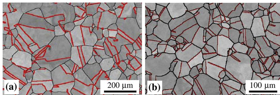
Fig. 1. Microstructure of the Ni–30%Fe alloy for different roughing temperatures: (a) 1200 °C, (b) 1000 °C. The red and black lines represent annealing twin and high angle grain boundaries, respectively. (For interpretation of the references to colour in this figure legend, the reader is referred to the web version of this article.)
