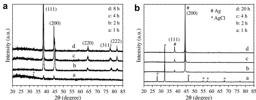
Fig. 1. XRD pattern of silver nanostructures synthesized using different  $\text{NaCl}$  concentrations: (a) 0.2 mM, (b) 20 mM.
