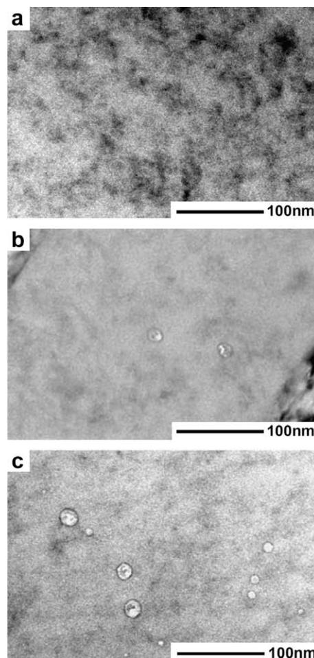
Fig. 1. TEM images of various Cu films aged for 30 min at  $400^\circ C$ : (a) Cu foil (A), (b) electroplated Cu film without SPS (B), and (c) with SPS (D).
