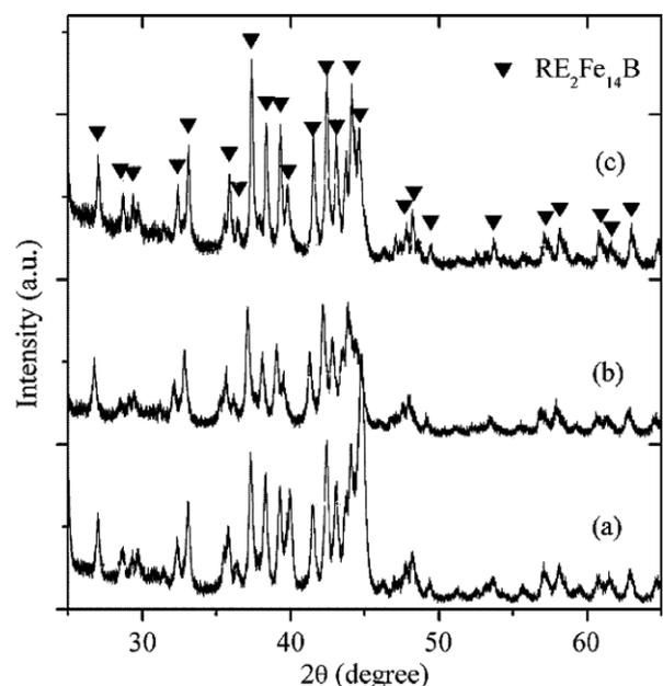
Fig. 1. X-ray diffractograms for: (a)  $\text{Nd}_{12}\text{Fe}_{82}\text{B}_6$ , (b)  $\text{RE}_{12}\text{Fe}_{78}\text{B}_{10}$ , and (c)  $\text{RE}_{12}(\text{Fe}_{0.9}\text{Co}_{0.1})_{76}\text{Zr}_2\text{B}_{10}$  alloys.
