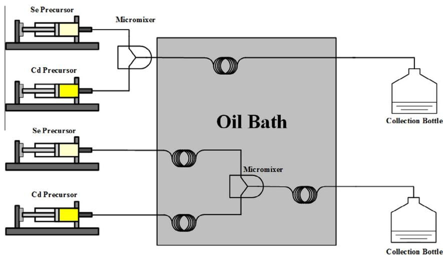
**Fig. 1.** Schematic diagram of two microfluidic methods for CdSe quantum dots synthesis.
