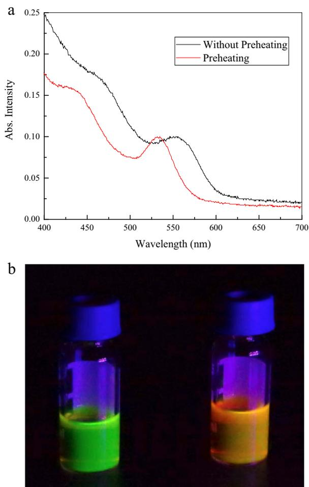
**Fig. 2.** CdSe quantum dots synthesized at 270 °C for 40 s with or without the preheating process. (a) UV-Vis. spectra and PL. spectra of the two samples. (b) A photograph of these two samples under a UV lamp. The left one was synthesized from preheated precursors, and the right one was synthesized from room-temperature precursors.
