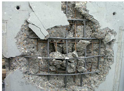
(a) without near-surface steel fabric reinforcement
