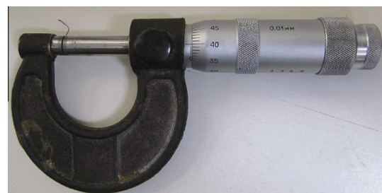
Fig. 2. Characterization of fibers: diameter measurement by a micrometer.
