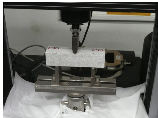
Fig. 1. A specimen during the three point flexural test.
