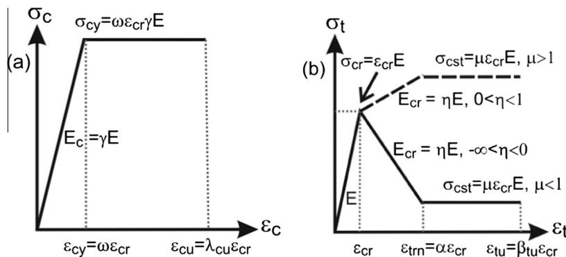
**Fig. 1.** Full option material models for both strain-hardening and strain-softening FRC: (a) compression model; and (b) tension model [22,23].
