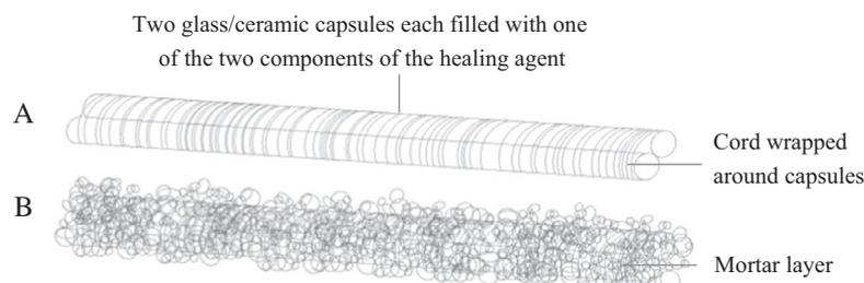
Fig. 1. Protection of the short glass and ceramic capsules by winding them with a cord (A) and providing a tiny mortar layer (B).
