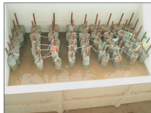
(b) Test-specimens in exposure tank.
