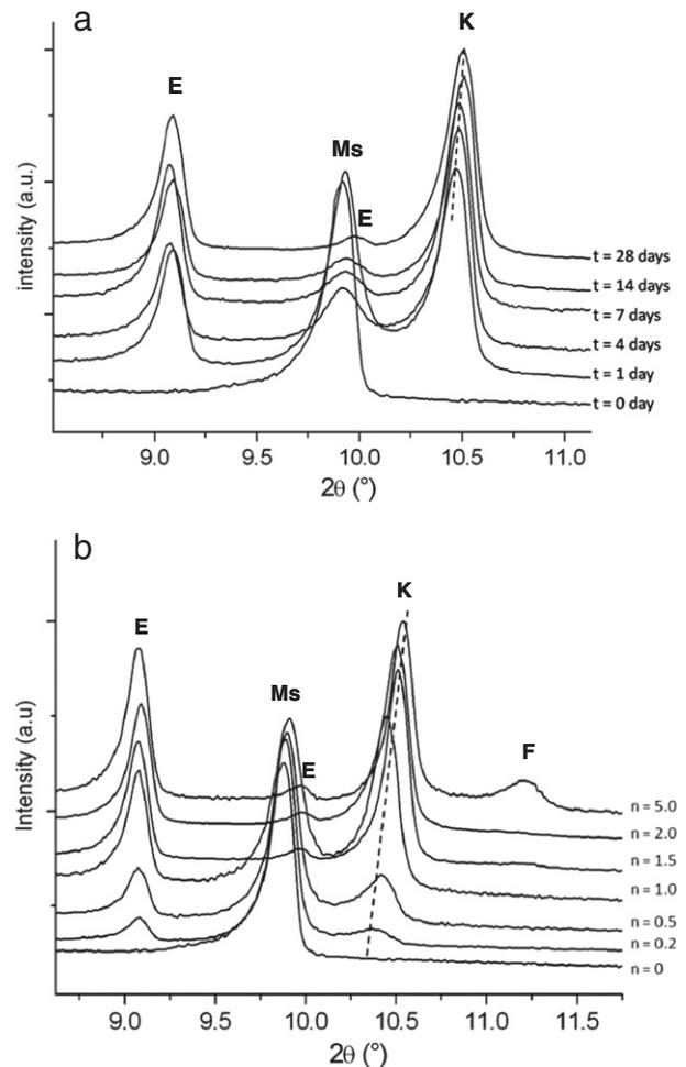
Fig. 1. XRPD patterns recorded after sorption tests with chloride anions (zoom on (001) reflexions). Influence of the reaction time (a) and of the initial chloride concentration (b) on the phase assemblage. Hydrates are labelled: Ms (calcium monosulfoaluminate hydrate), K (Kuzel's salt), E (ettringite) and F (Friedel's salt).  $n$  indicates the initial chloride/monosulfoaluminate molar ratio. The time series was performed at  $n = 2$ .
