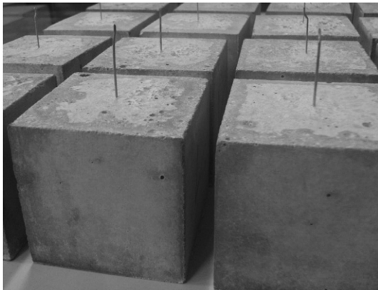
Fig. 1. Single fiber pullout specimens.
