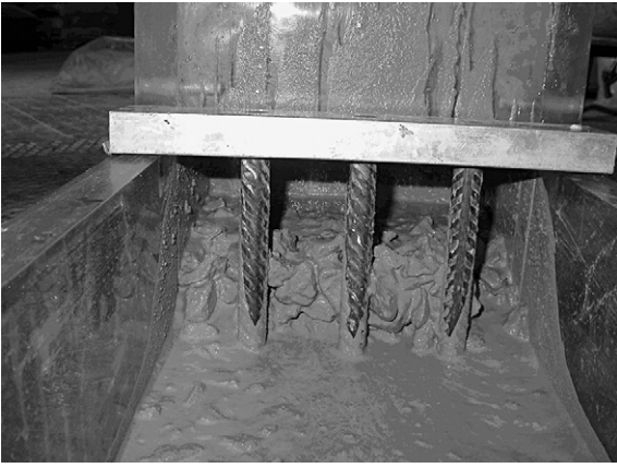
Fig. 1. Granular blocking during a L-Box test on SCC (from [4]).
