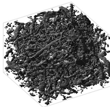
Fig. 1. 3D reconstruction of the soil core by serial sectioning. The pixel resolution is 100 \mu\text{m} (adapted from [9,10]). The region of interest is 1 mm in dimension.
