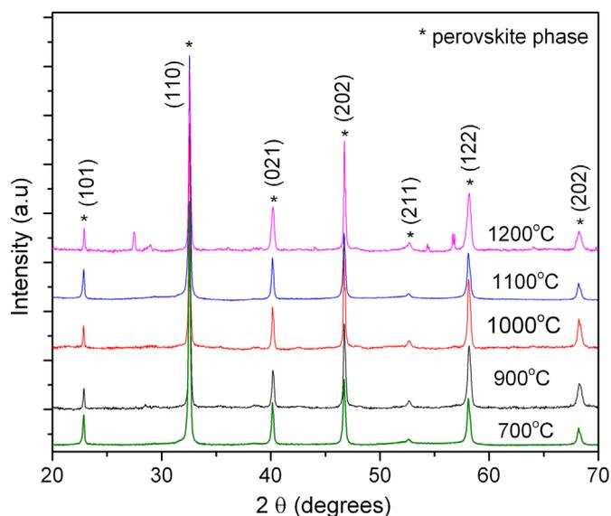
Fig. 2. XRD of BNT powder calcined at 700 °C and sintered pellets at 900 °C, 1000 °C, 1100 °C and 1200 °C.
