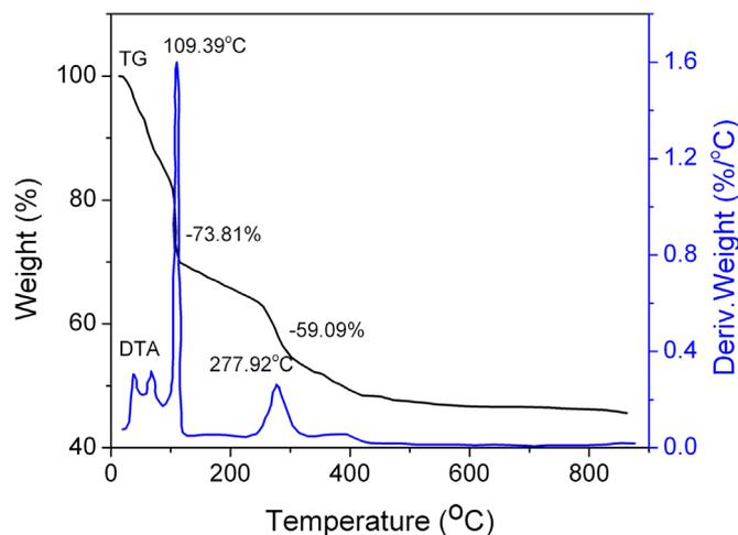
Fig. 1. TG and DTA curves of NBT dried xerogel.
