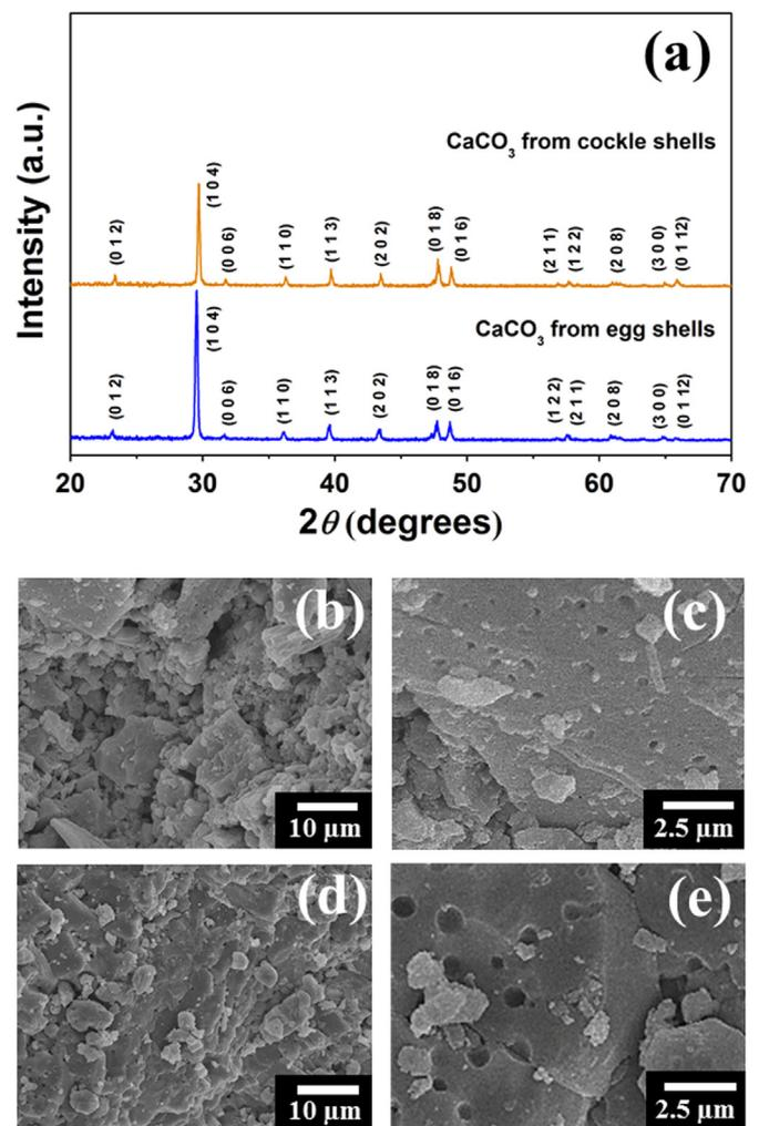
**Fig. 1.** (a) XRD patterns of  $\text{CaCO}_3$  powders synthesized from different natural raw materials, (b, c) SEM micrographs of  $\text{CaCO}_3$  powders synthesized from the egg shells (at low and high magnifications, respectively), and (d, e) SEM micrographs of  $\text{CaCO}_3$  powders synthesized from cockle shells (at low and high magnifications, respectively).
