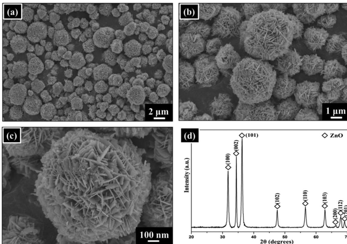
**Fig. 1.** FESEM images and XRD pattern of ZnO structures synthesized from the reaction of 0.1 M zinc acetate, 0.24 M citrate and 0.5 M sodium hydroxide at room temperature under stirring for 2 h. (a, b, and c) FESEM images of the sample, (d) XRD pattern of the sample.
