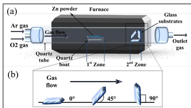
Fig. 1. Schematic of the set-up used for the growth of ZnO-Ts by thermal evaporation method.
