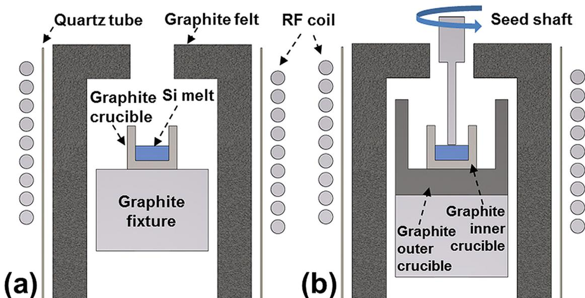
Fig. 1. The layout of experiments of (a) Si melting test and (b) SiC crystal growth by the TSSG method.
