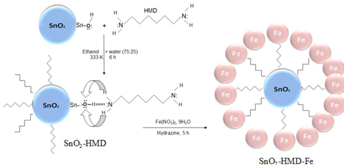
Scheme 1. Synthetic strategy towards  $\text{SnO}_2$ -HMD-Fe for hydrogen capture.
