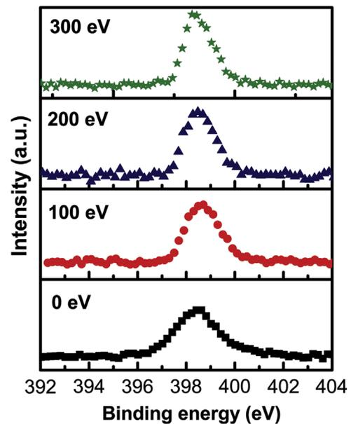
Fig. 2. The XPS spectra of N 1s on the surface of the BN films with different assisted ion-beam energy bombardments.
