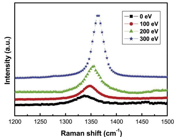
Fig. 3. Raman spectra of the BN films (a) without assisted ion-beam bombardment, (b) with 100 eV assisted ion-beam bombardment, (c) with 200 eV assisted ion-beam bombardment, and (d) with 300 eV assisted ion-beam bombardment.
