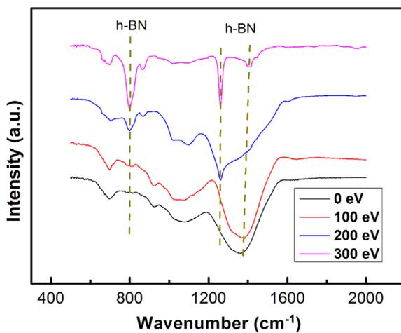
Fig. 1. FTIR spectra of (a) without assisted ion-beam bombardment, (b) with 100 eV assisted ion-beam bombardment, (c) with 200 eV assisted ion-beam bombardment, and (d) with 300 eV assisted ion-beam bombardment.
