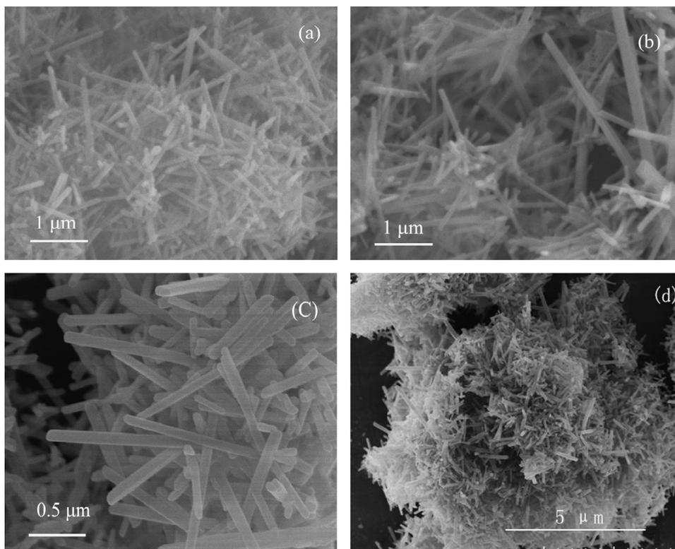
Fig. 2. SEM images of samples (molar ratio of  $\text{H}_3\text{BO}_3$ :AACH=1:2.5) calcined at  $1100^\circ\text{C}$  for different time (x): (a)  $x=2.5$  h, (b)  $x=3.0$  h, (c)  $x=4.0$  h.
