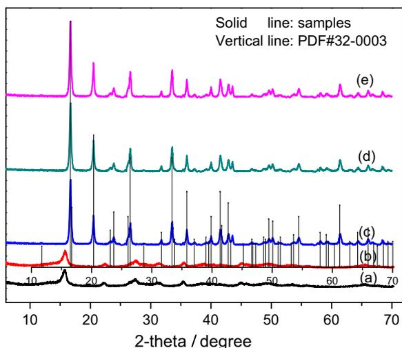
Fig. 1. XRD patterns of PDF#32-0003 and samples: (a) AACH, (b) precursor (molar ratio of AACH: $\text{H}_3\text{BO}_3$ =2.5:1) and samples calcined at  $1100^\circ\text{C}$  for different time (x): (c)  $x=2.5$  h; (d)  $x=3.0$  h; (e)  $x=4.0$  h.
