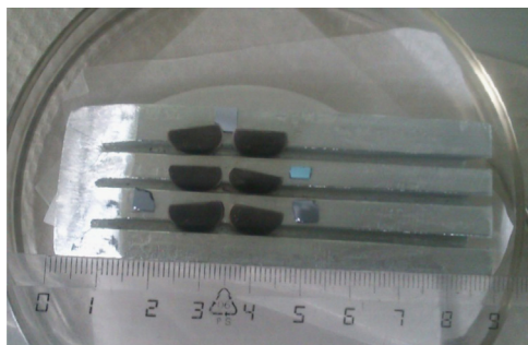
Fig. 1. Pieces of silicon wafer and SiC samples (tablets) in holder rabbets prepared for ALD.
