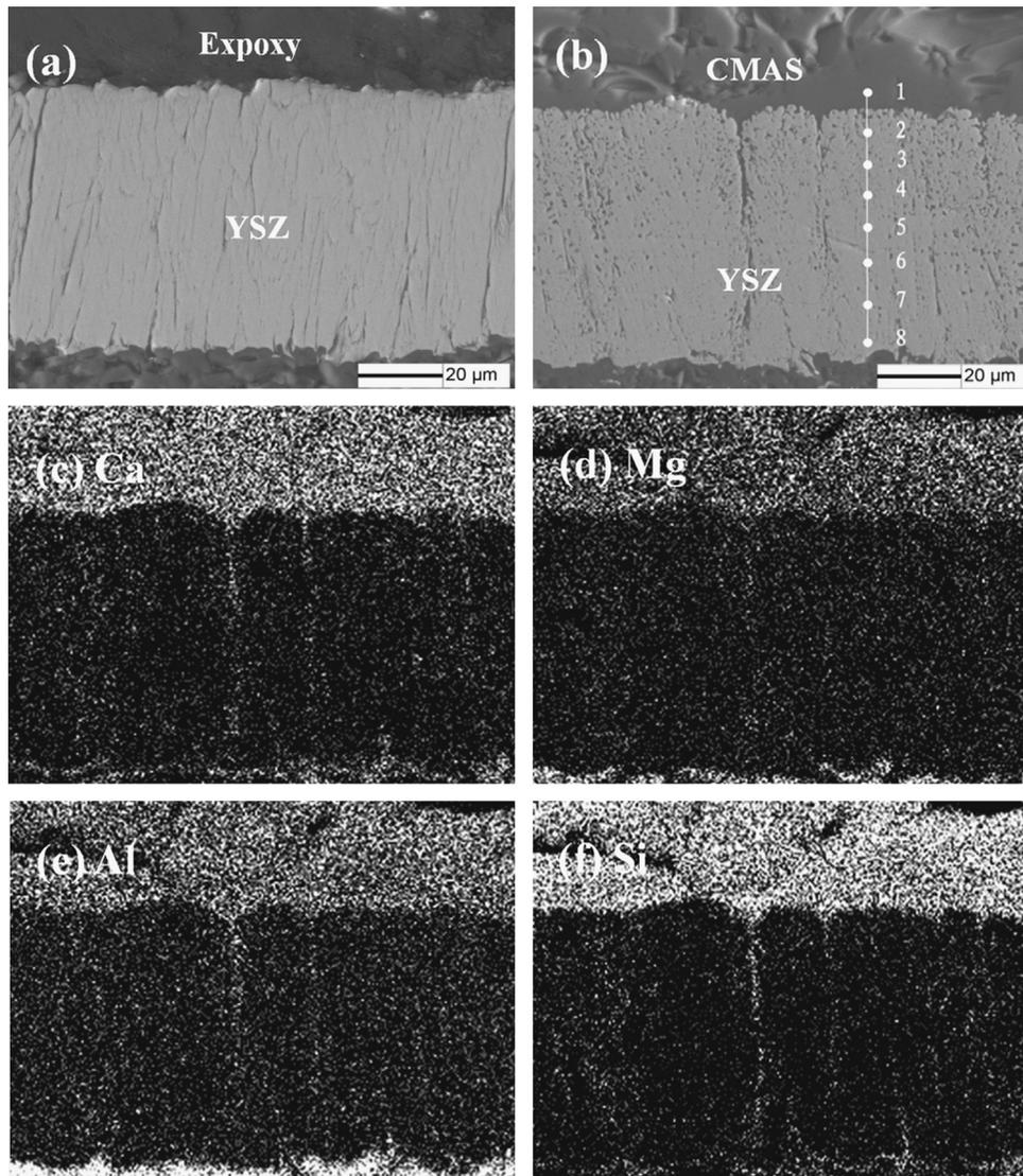
Fig. 1. Cross-section images of YSZ coatings after heat treatment at 1250 °C for 4 h without (a) and with (b) CMAS deposits, (c)–(f) show the element maps of the YSZ coating after CMAS attack.
