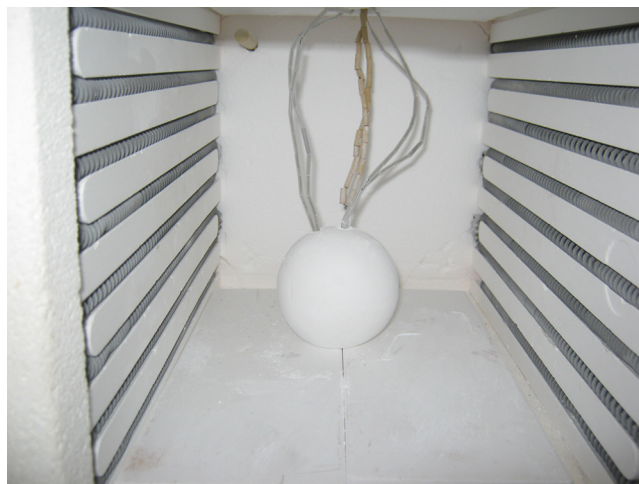
Fig. 1. The setting of alumina sphere ( \varnothing \approx 75 mm) and thermocouples in a furnace.
