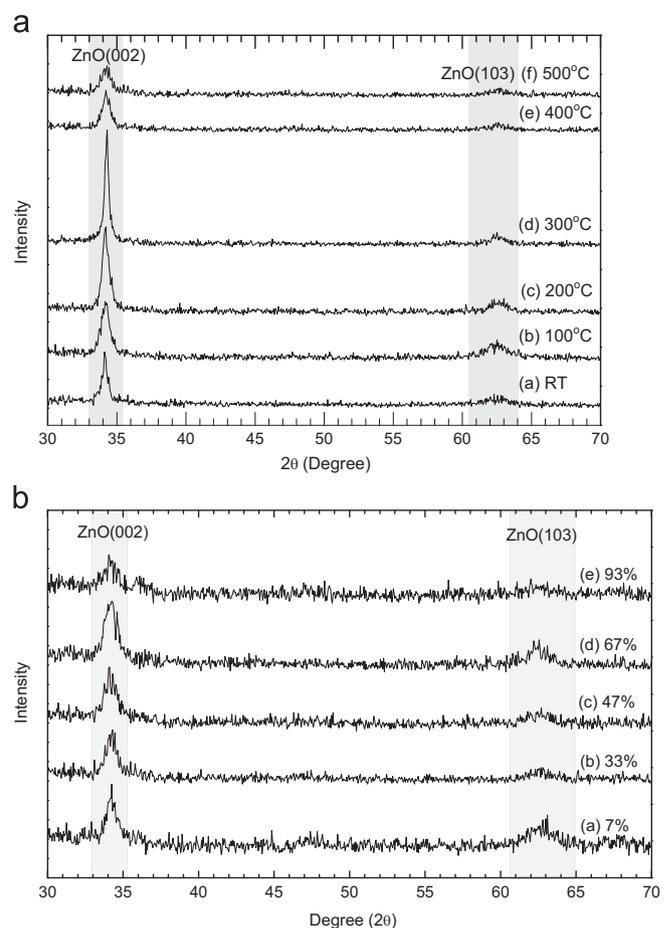
Fig. 1. (a). Phase analysis based on the XRD patterns of ZnO films deposited at 33% oxygen percentage and under various growth temperatures (RT to 500 °C). Fig. 1(b). Phase analysis based on the XRD patterns of ZnO films deposited at growth temperature of 500 °C and under varying oxygen percentages (7–93%).
