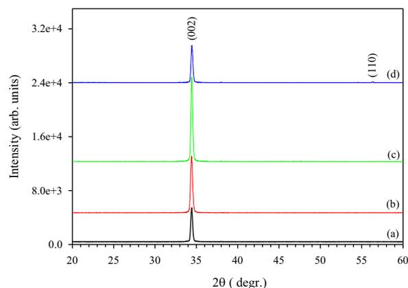
Fig. 1. XRD patterns of undoped ZnO (a) and Mn-doped ZnO nanorods (grown into the honeycomb lattice) annealed at 500  $^{\circ}\text{C}$  (b), 600  $^{\circ}\text{C}$  (c), 700  $^{\circ}\text{C}$  (d) for 8 h.
