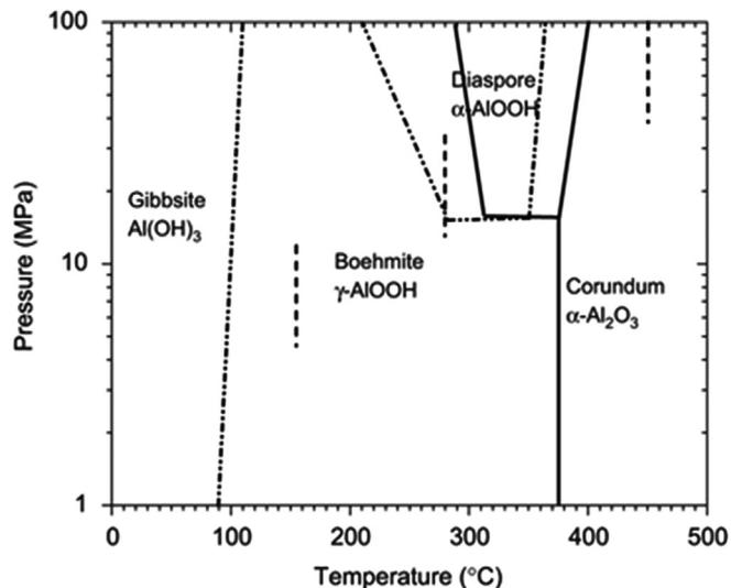
Fig. 1. Hydrothermal Al<sub>2</sub>O<sub>3</sub>–H<sub>2</sub>O phase diagram from [1] with permission © 2009, The American Ceramic Society.
