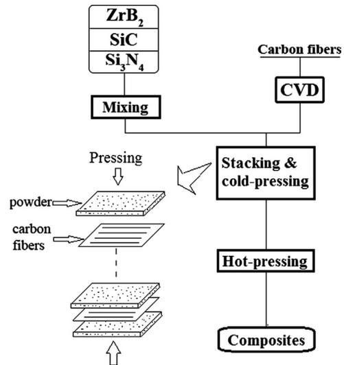
Fig. 1. Illustration of the preparation process of unidirectional carbon fibers reinforced  $ZrB_2$ –SiC based composite.
