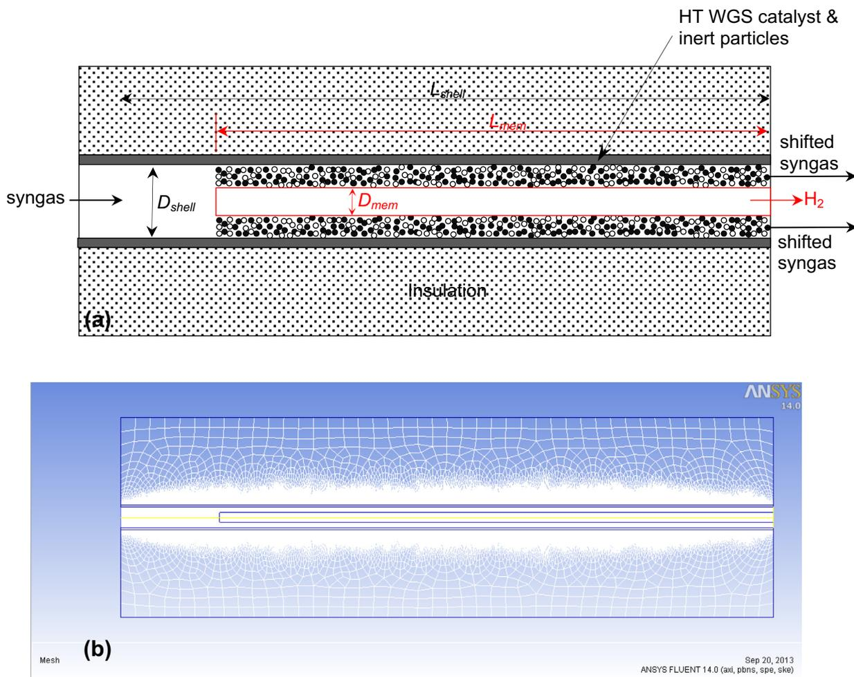
Fig. 1. (a) Schematic diagram of catalytic membrane reactor used in this study. (b) Geometry and mesh of CMR used for 2D-axisymmetric model.
