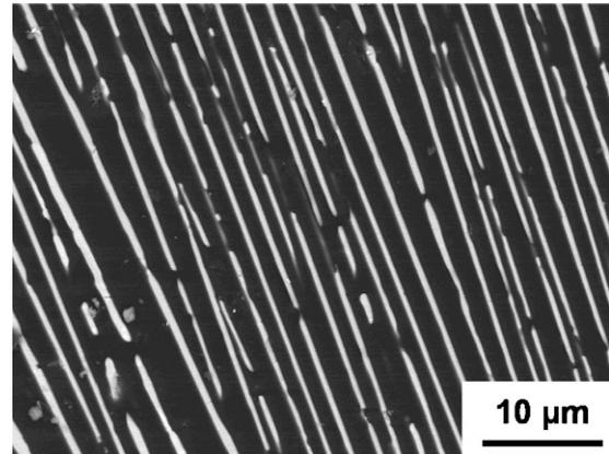
Fig. 1. Microstructure of the directionally solidified eutectic  $B_4C$ – $TiB_2$  alloy.
