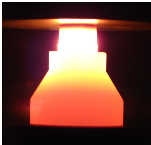
Fig. 2. Real-time colour distribution of graphite mould during the sintering. Note that the white, yellow and red colour represent high, intermediate and low temperature respectively. (For interpretation of the references to colour in this figure legend, the reader is referred to the web version of the article.)
