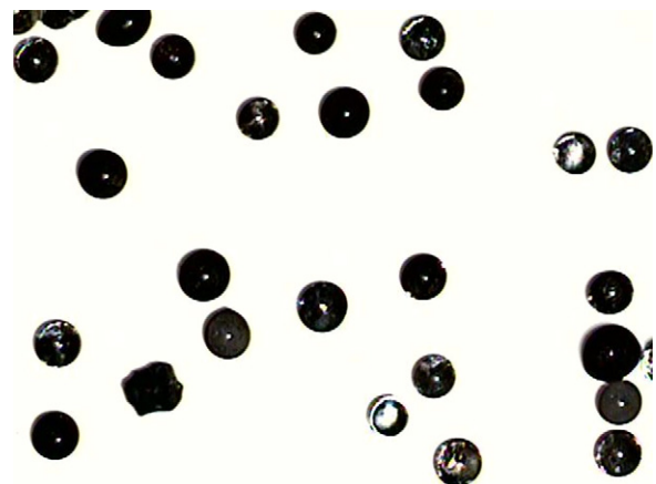
Fig. 1. Morphology of microspheres obtained at gases feeding flow of 2 L/min (1:1Ar:He rate) and 1000 A.
