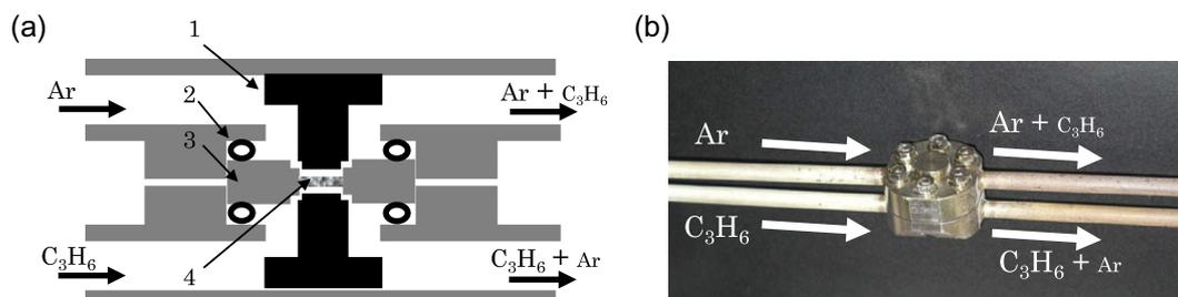
**Fig. 1.** (a) The Wicke–Kallenbach-type counter-current diffusion cell: (1) gas current control section, (2) metal O-ring, (3) SUS section to fix to metal mesh, and (4) simulated washcoat layer. (b) Photograph of the diffusion cell.
