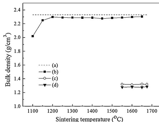
Fig. 2. (a) Theoretical density of low cristobalite, and measured bulk densities of the sintered samples from (b) uncalcined SiO<sub>2</sub> amorphous raw powder, and those calcined at (c) 1150, and (d) 1200 °C for 3 h.
