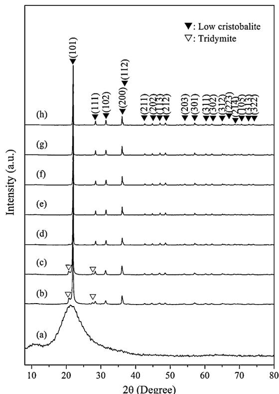
Fig. 3. XRD patterns of samples from SiO<sub>2</sub> raw powder sintered at (a) 1100, (b) 1150, (c) 1200, (d) 1250, (e) 1350, (f) 1450, (g) 1550, and (h) 1650 °C for 3 h.
