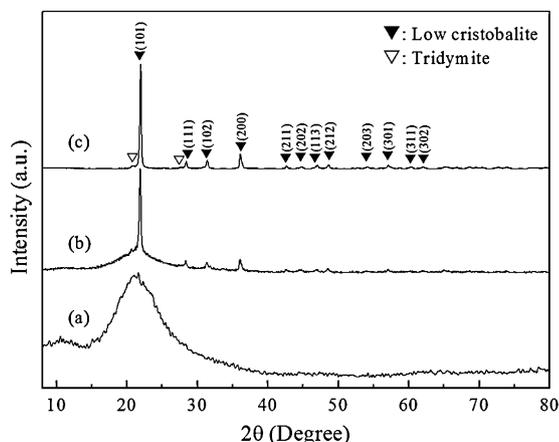
Fig. 1. XRD patterns of (a) SiO<sub>2</sub> amorphous raw powder and powders calcined at (b) 1150, and (c) 1200 °C for 3 h.
