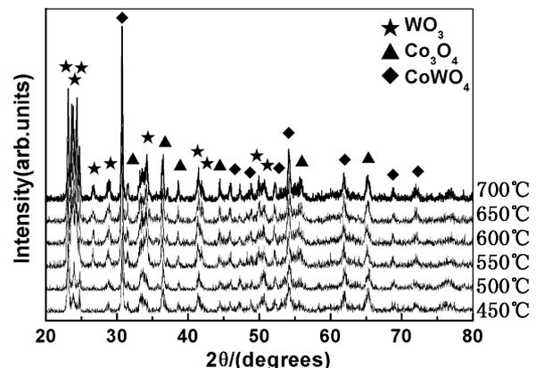
Fig. 2. XRD patterns of the surface of the ultrafine WC–10Co-cemented carbide, oxidized at different temperatures.
