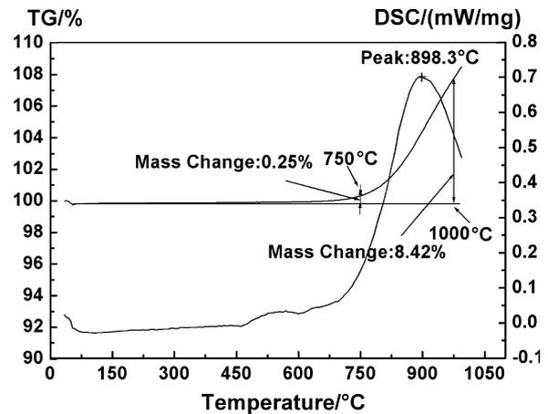
Fig. 1. DSC/TG pattern of ultrafine WC–10Co-cemented carbide from room temperature to 1000 °C in air.
