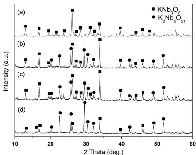
Fig. 3. XRD patterns of the obtained products with different weight ratios  $R$  of  $\text{KCl}$  to  $\text{K}_2\text{SO}_4$ . (a)  $R = 0.5$ ; (b)  $R = 1$ ; (c)  $R = 2$ ; (d)  $R = 4$ .
