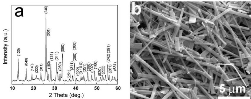
Fig. 1. (a) XRD pattern and (b) typical SEM image of the as-synthesized  $\text{KNb}_3\text{O}_8$  nanobelts.
