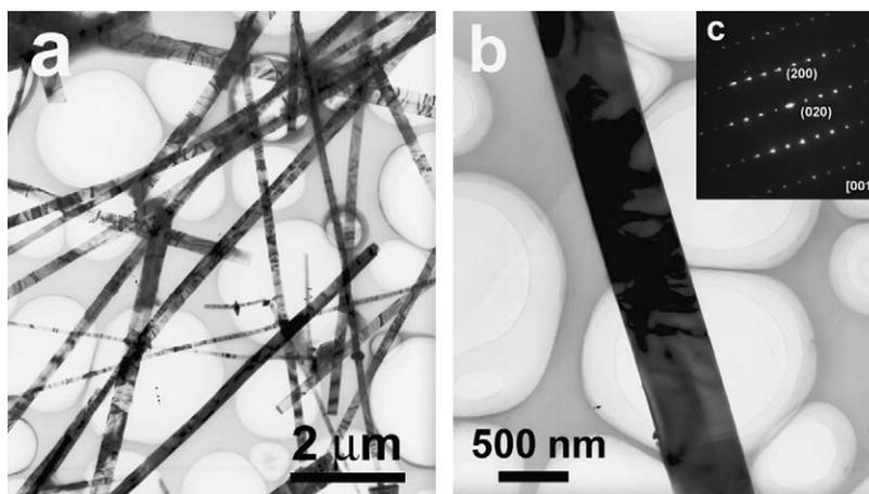
Fig. 2. (a) TEM image of the as-synthesized  $\text{KNb}_3\text{O}_8$  nanobelts showing their general morphology, (b) TEM image of an individual nanobelt and (c) corresponding SAED pattern taken from the selected nanobelt.
