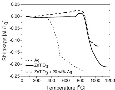
Fig. 1. Shrinkage curves of Ag, ZnTiO<sub>3</sub> and their composite.
