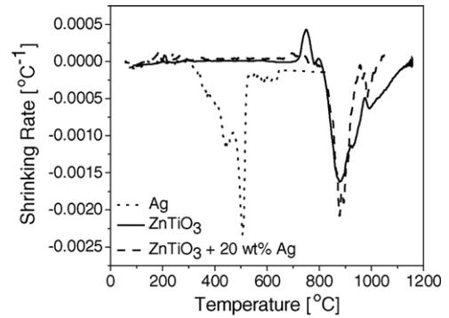
Fig. 2. Shrinking rate curves of Ag, ZnTiO<sub>3</sub> and their composite.
