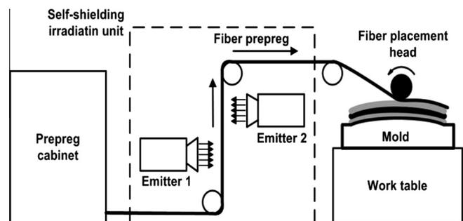
Fig. 1. Illustration of low-energy EB cured thermoset tape placement process.
