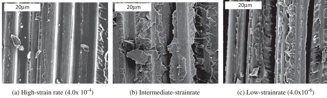
**Fig. 1.** SEM photograph of failure surface for transverse tensile test with various strain rate: Interface failure appears at high-strain rate and matrix failure appears at low strain rate.
