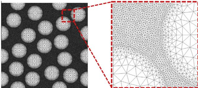
**Fig. 2.** Periodic unit cell with mesh and magnified one: triangle quadratic element is used, fine mesh is adopted for matrix part and near interface, no volume cohesive element is inserted at every interface. (For interpretation of the references to color in this figure legend, the reader is referred to the web version of this article.)
