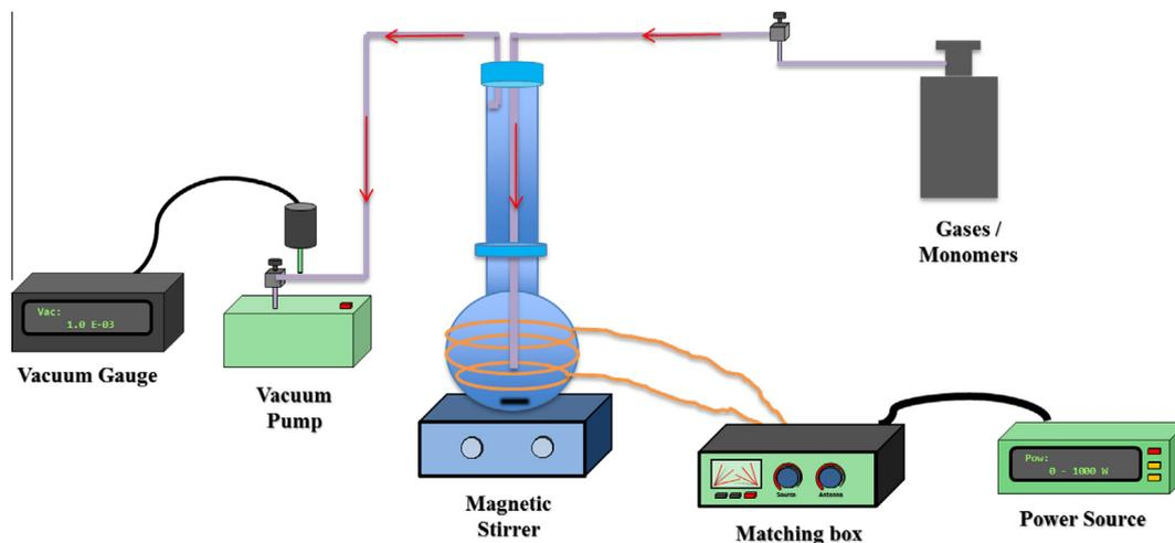
Fig. 1. Schematic diagram of the stirring plasma system. (For interpretation of the references to colour in this figure legend, the reader is referred to the web version of this article.)
