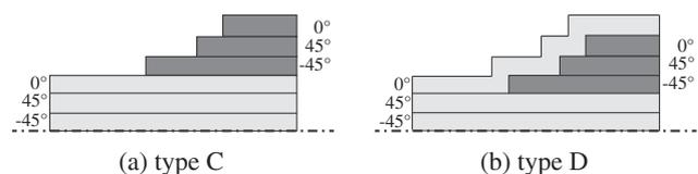
Fig. 1. Symmetric half of the locally reinforced specimen types.
