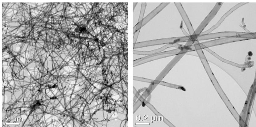
Fig. 1. TEM micrographs showing morphologies of CNTs.
