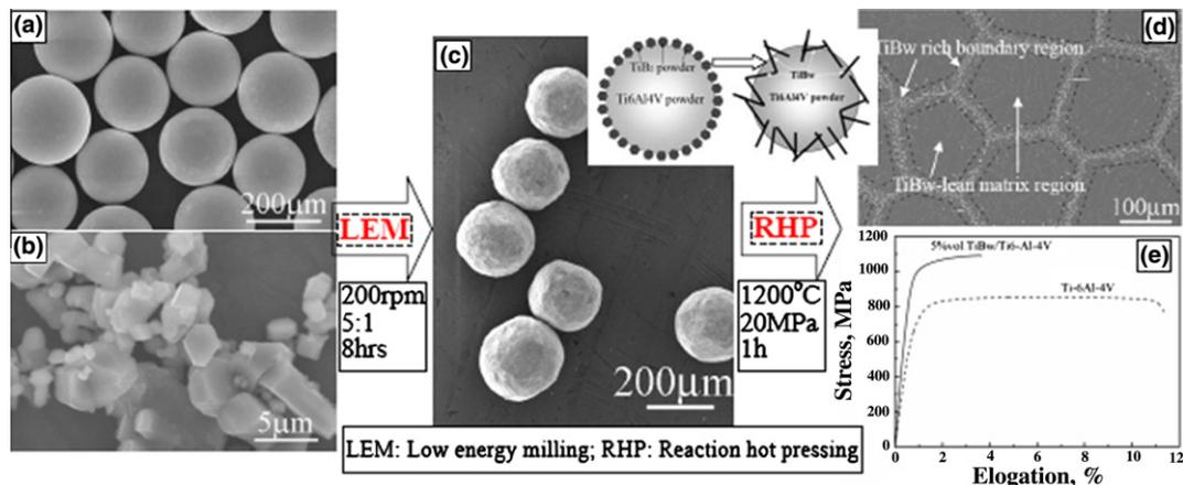
Fig. 1. SEM micrograph of *in situ* 5 vol.%TiBw/Ti64 composite with a quasi-continuous network microstructure [12]. (For interpretation of the references to color in this figure legend, the reader is referred to the web version of this article.)
