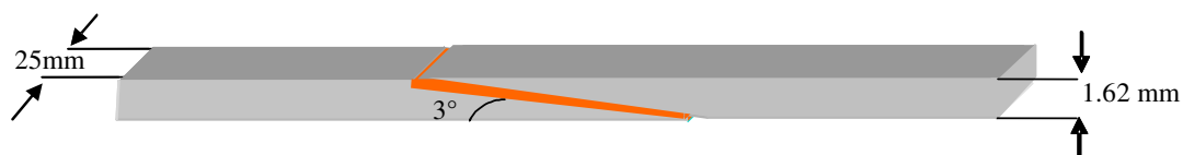
Fig. 2. Mini-scarf configuration used to examine adhesive shear strength of composite bonded joints.
