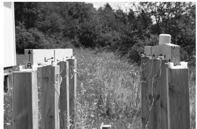
Fig. 1. Photograph of the untreated (left) and treated (right) specimens at the beginning of the 1-year exposure test. The “R” and “L” arrows denote the radial and longitudinal directions, respectively; the tangential direction is perpendicular to the radial direction on the front face. The tangential surface is on the top of the board and cannot be seen in these images.
