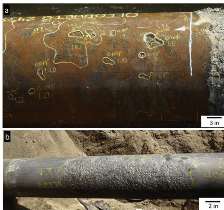
Fig. 1. Photographs of two excavated pipelines where corrosion defects are found (a) mainly as isolated features in an excavation ditch in a 24-in diameter pipeline, and (b) grouped in a cluster in a section of a 6-in diameter pipe.
